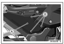
A. Air Cleaner Element Cap B. Mounting Screws
