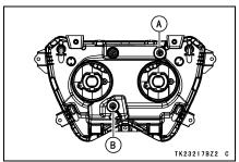
A. Horizontal Adjuster B. Vertical Adjuster
