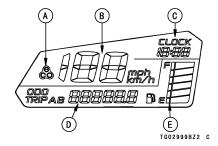
When the ignition switch is turned on, all LCD segments are displayed with opening display functions for few seconds, then the multifunction meter turns to operational mode.
