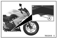
A. Engine Oil Drain Bolt
