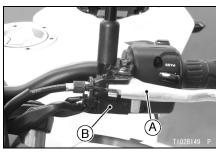
A. Clutch Lever B. Starter Lockout Switch
