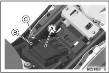
A. Relay Assy B. Battery Cover C. Cover Screw
