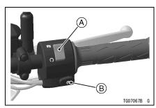
A. Engine Stop Switch B. Starter Button
