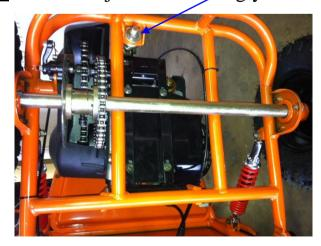
3. After the go-kart has been driven for a while, the <u>drive</u> <u>chain on clutch</u> will be loosen and should be readjusted. At first, <u>four bolts</u> fixing the engine on mount plate have to be loosen until the engine can be moved. Then, adjust the <u>chain adjusting</u> <u>bolt at the front side of engine</u> to tighten the chain to an appropriate tension. At last, after adjusting screw the four bolts tightly.
