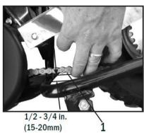
2. If after step. 1 tightening the nut of chain adjustor the chain is still too loose or too tight, another nut at the underpart of chain adjustor must be adjusted accordingly.
